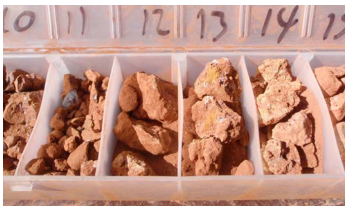
Figure 3 – Bauxite chips from depth interval 10 – 15m
