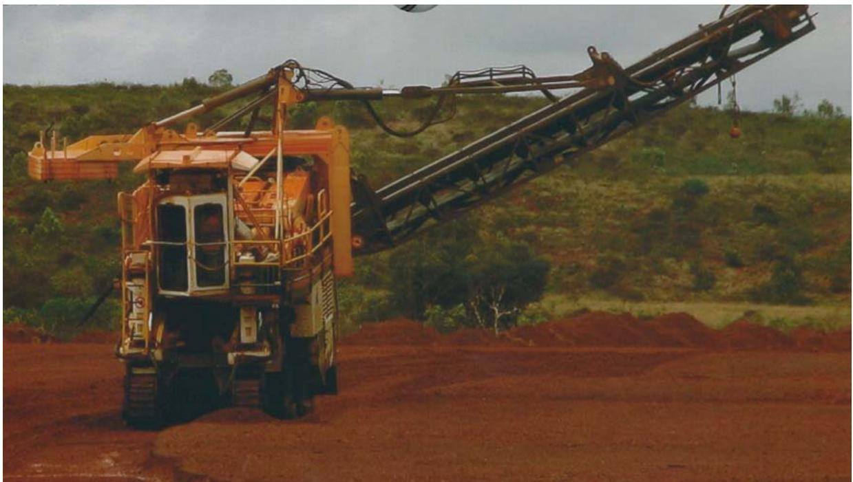
Figure 4: Wirtgen Surface Miner
